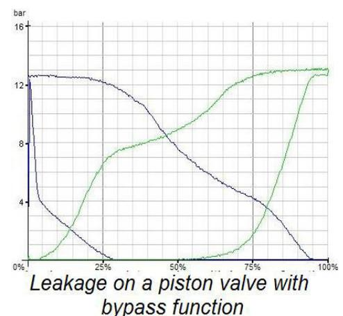
Possible valve gear faults, leaks, valve damage as well as the correct dimensions of the clearance volumes can be reliably read from the diagrams.
